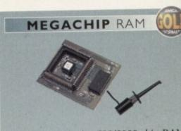
Increase your Amiga 500/2000 chip RAM to a total of 2MB. MegaChip does this by using its own 1MB of RAM and drawing extra memory from any other RAM you have installed in your Amiga. No soldering required.
